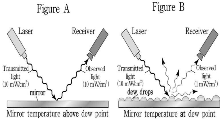
Figures A and B demonstrate how dew point is measured by a dew point hygrometer. In Figure A, light is transmitted from a laser and ① reflected off the mirror onto a receiver that measures the intensity of the observed light. When the
